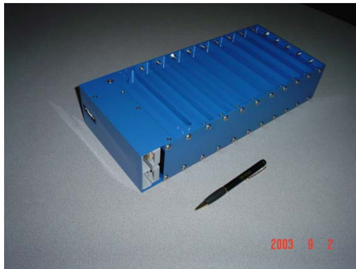
Figure 11. Nominal 6 Ah 40 Volt Deliverable to SNL
