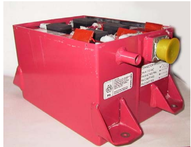
Figure 4 Existing Lead Acid Battery for the F-16
